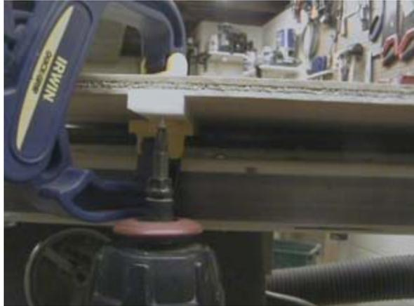
After the screw is attached, I push the sled forward and attach the screw at the other end. All while the factory edge is against the fence and the runner is still in the miter slot.
