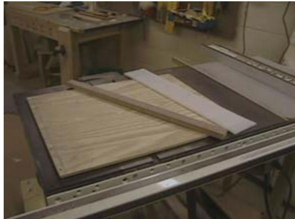
My first step is to cut the UHMW to use as a runner on the base of the sled. The UHMW is easy to shape and cut and also decreases any friction between the sled and the table top.
