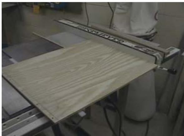
The runner is pulled forward and clamped to the plywood. This allows me to attach the screw securely in place.
