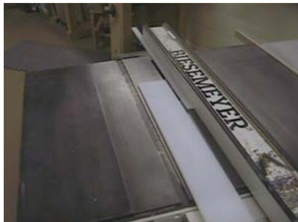
Once the piece of UHMW is cut to the correct width, I clean up the edges with a block plane to ensure it rides in the miter slot with ease. But at the same time there should be very little if any side to side movement.
