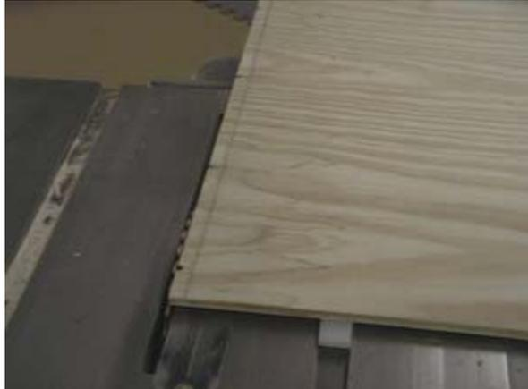
With the new parallel edge it's time attach the fence. I start by screwing the fence with one screw. This gives me a pivot point from which I can make adjustments. So the next step is to ensure that the fence is perfectly perpendicular to the new parallel edge. This can be achieved with either a very reliable carpenter's square or a little geometry. Once it's squared drive a few more screws to secure it in place.
