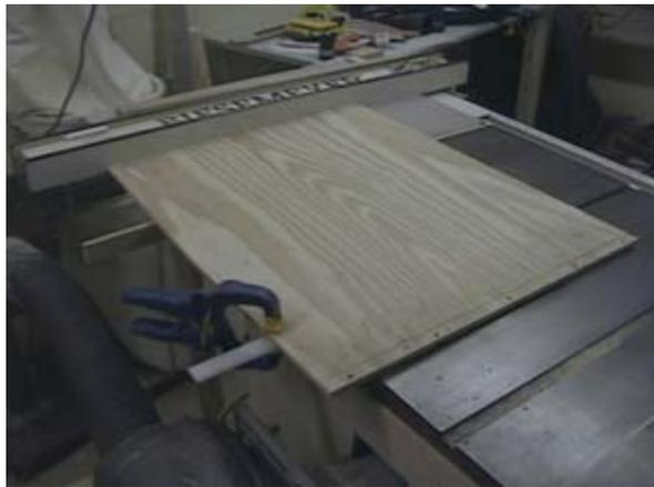
Once the front and rear screws are in place I can securely attach the middle screw and then here I added a few extra (a little overkill actually).
