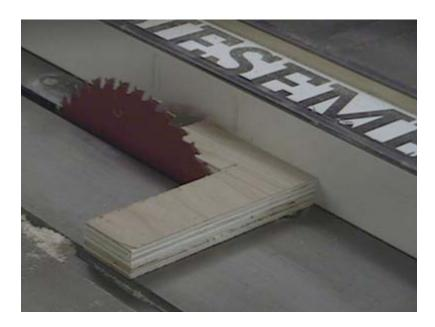
Here are the finished jigs in action. To help keep the L's from getting glued into place during the glue up, I took them over to the miter saw and cut the heel off.
