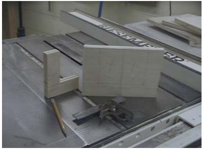
The first step is to make sure that the scrap is square on at least two edges, that way all your cuts from that point on are parallel.
