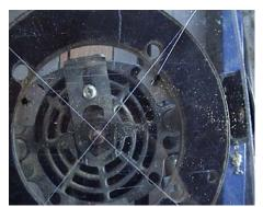
With a ¼ inch straight bit in the router I lay the plate With the center of the X directly over the center of the bit.
