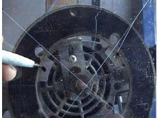
With a felt tip pen I mark a dot directly over the mounting holes on the base. Keeping the X centered over the bit.
