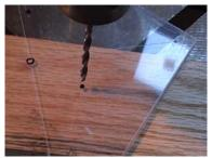
Then with a smaller bit I drill for the mounting screws.
