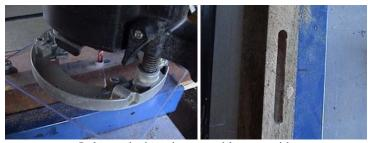
I clamped a board to my table saw. with a bearing snug against each side of the board
