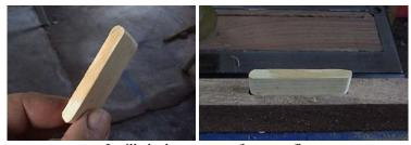
I milled a loose tenon for a test fit.
