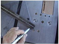
I marked a dot ¾ of an inch from the corner being careful to stay on the line.
