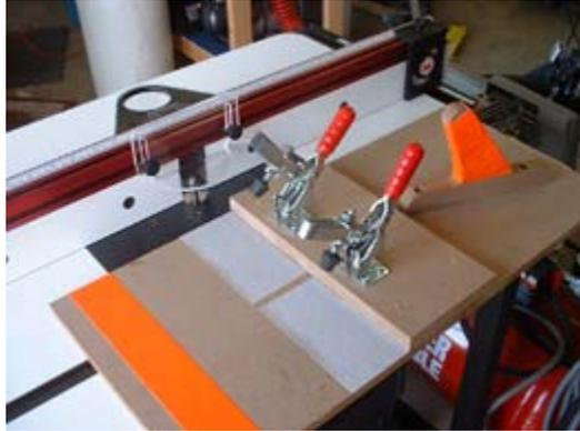
Two more features to point out are the sandpaper under the toggle clamps. The purpose of the sandpaper is to increase surface friction and thus increase clamping strength. A very crucial feature as the component enters the spinning cutter. The next feature is the orange tape. This is a safety reminder of where it's best not to have your hands and fingers during the cutting action.
