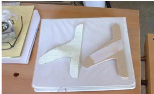
The handle is easily made from a couple of scraps of MDF and custom fitted for your hand. Here we see the progression from paper pattern to template and soon on to the MDF.
