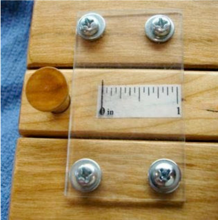
After trimming the ruler to size it was clear coated with spray shellac and glued in place on the registration bar. The Plexiglas cover is from an old broken drafting triangle.
