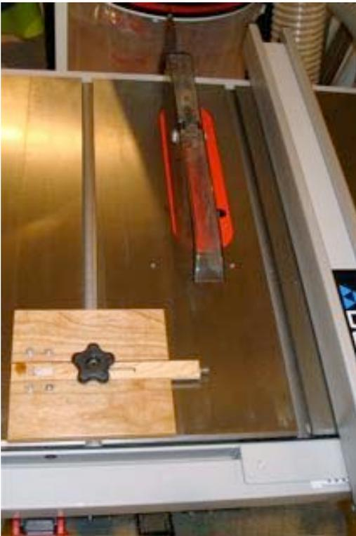
With your stock against the rip fence, slide the fence until the stock is just touching the socket screw. The saw is now set to rip thin stock of the desired thickness. Now all you have to do is move the fence over each time, touching the socket screw, and rip another piece of stock of the same thickness.
