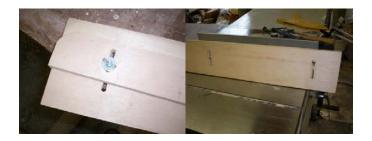
For the slots on the base piece, we're going to need to countersink the slots to accommodate the carriage bolt's head so that it will ride smoothly across your tabletop.
