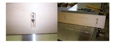
This countersinking can either be done freehand with your router (please be extra careful so it doesn't get away from you) or with a series of cuts using a forstner bit. Either way, make these cuts deep enough for the carriage bolt.
