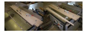
You're finally result will be a nicely tapered component cut to the exact angle and size that your project requires! Just keep the fence in place and you're ready to go again!
