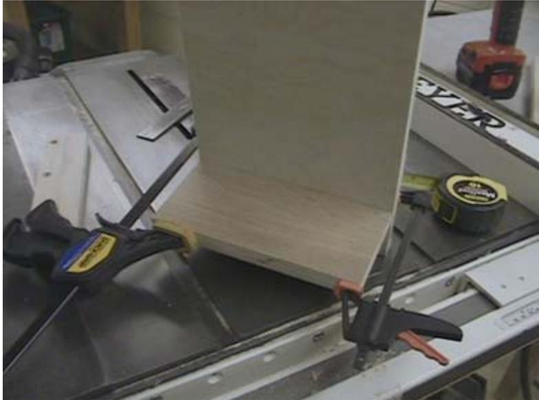
The first screw to be set is the middle screw. This gives me a chance to find the right level on the left and right before finishing.
