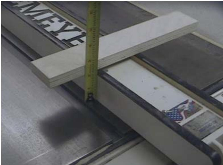
To help get an accurate measurement of the fence side, I rested a strip on the top of the fence and measured from the table top to the bottom of the strip. The main reason for this is that the fence side has a rounded edge treatment that made it difficult to determine the height without the reference edge for accuracy.
