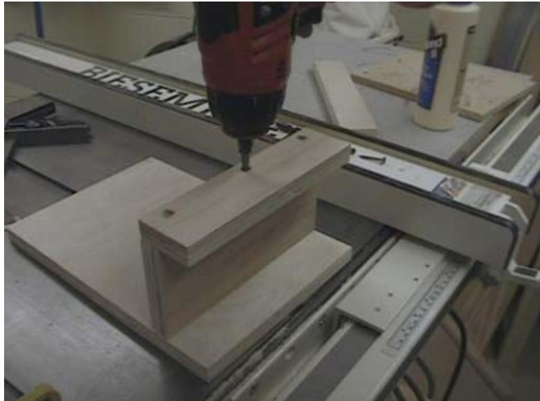
Step 7. The sacrificial fence is attached. I'm not worried about the appearance since it will be replaced from time to time. The main concern is to make sure the edge backing the component is square to the table. If it's not, your tenons won't be either.
