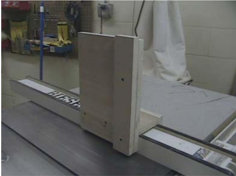
Here's the jig in action (not really, but it kind of looks like it doesn't it?) Some improvements on this basic design would include a handle on the bridge, and a modified clamp to hold the component tight to the jig.
