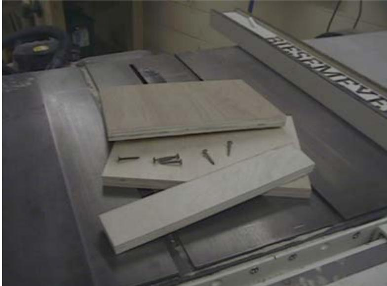
Step 1. The tenon jig rides on the fence, so the first step is to measure its height.
