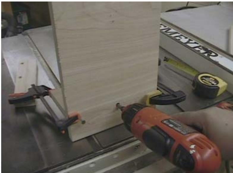
The same is true for the the short side. A bead of glue, some clamps and then the screws.
