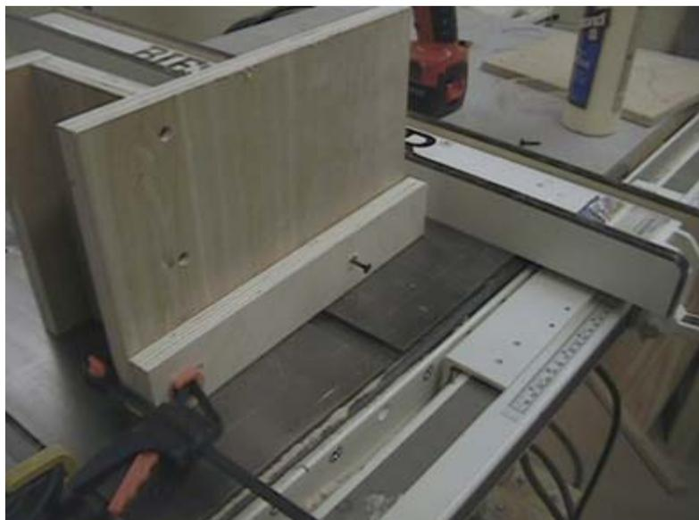
This is the completed jig. As you can see it rides on the fence. The key is to have a snug fit but yet it can move back and forth with slight effort. A little wax and it should be ready for action.
