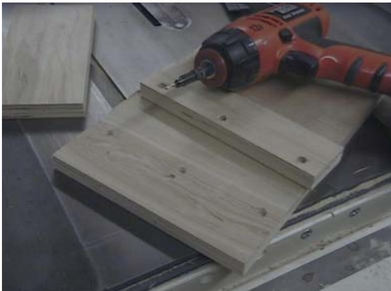
Countersinking the holes is critical to making sure the blade doesn't accidentally nick the screw heads.
