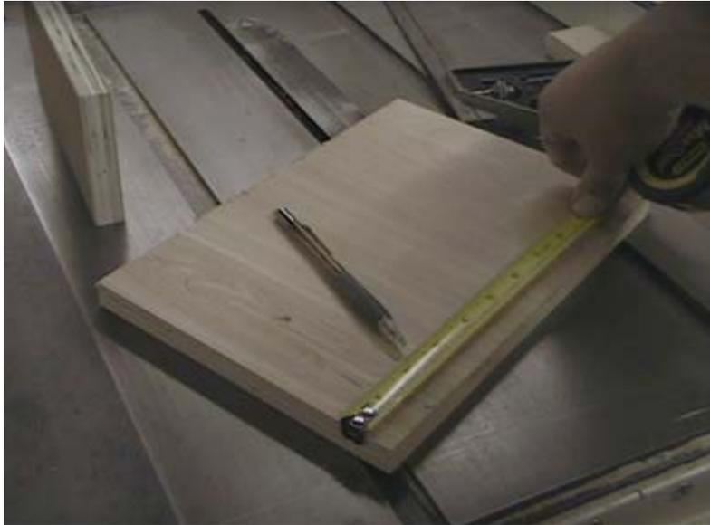
Step 5. The reference line I just drew, represents the bottom edge of the bridge. Since I know the thickness of the material I can determine the center line and then drill and countersink holes for the screws that will join the side to the bridge. Since I'm already drilling the tall side I went ahead and drilled the short side too. It's less critical about positioning the short side but I have the top of it flush with the bridge.
